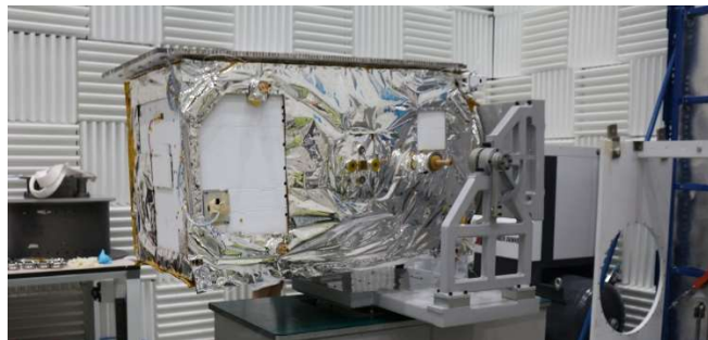
Fig. 5. The measurement of CoM of Taiji-1.
